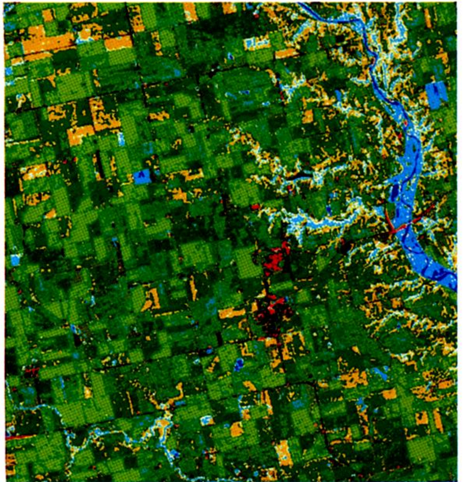
FIGURE 6. Portions of a Landsat scene before (left) and after (right) the application of 100 iterations of unsupervised ISODATA classification algorithm.
